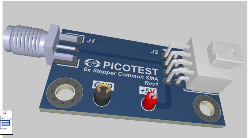
Figure 19: The S50COMMON common breakout board allow you to turn on and off all 6 switches to control a ‘full load’ current step.
