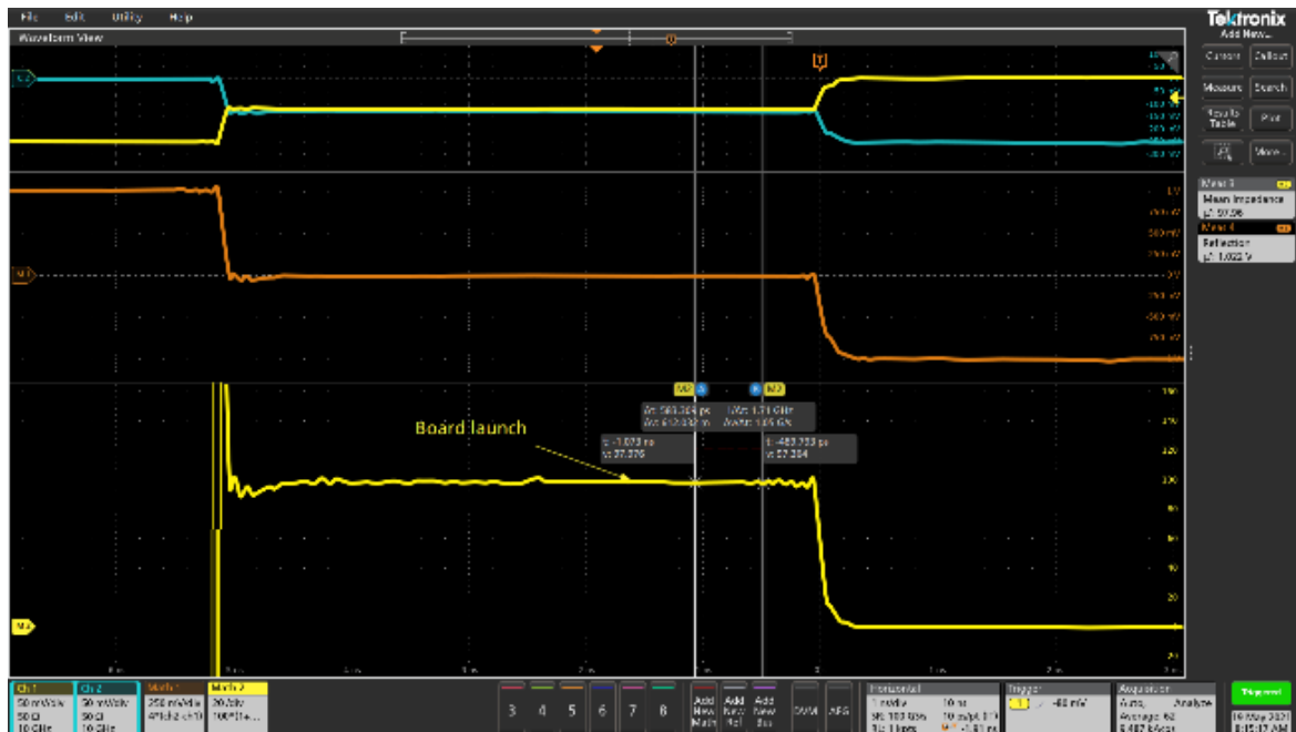
Figure 6: The P2103A recorded differential signal, gamma function and 100 Ohm measurement.
