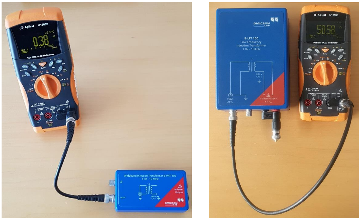
Figure 1: Measurement setup - DC resistance of input
