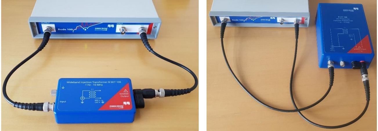
Figure 4: Measurement setup - check of frequency range
