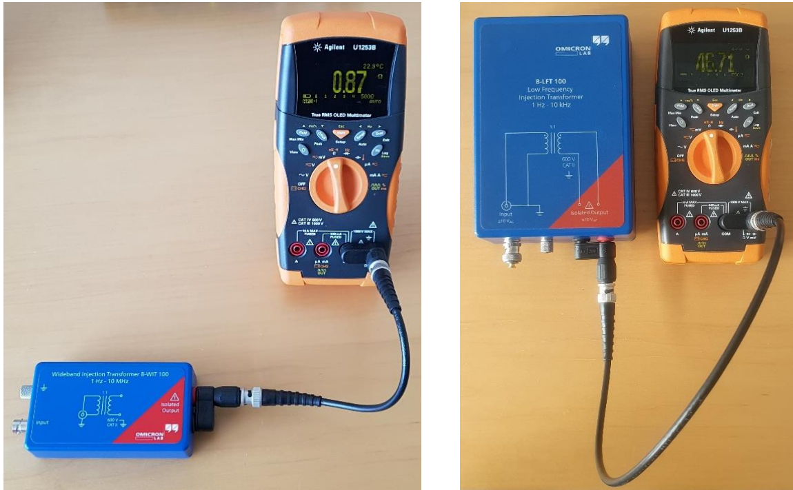
Figure 2: Measurement setup - DC resistance of output
