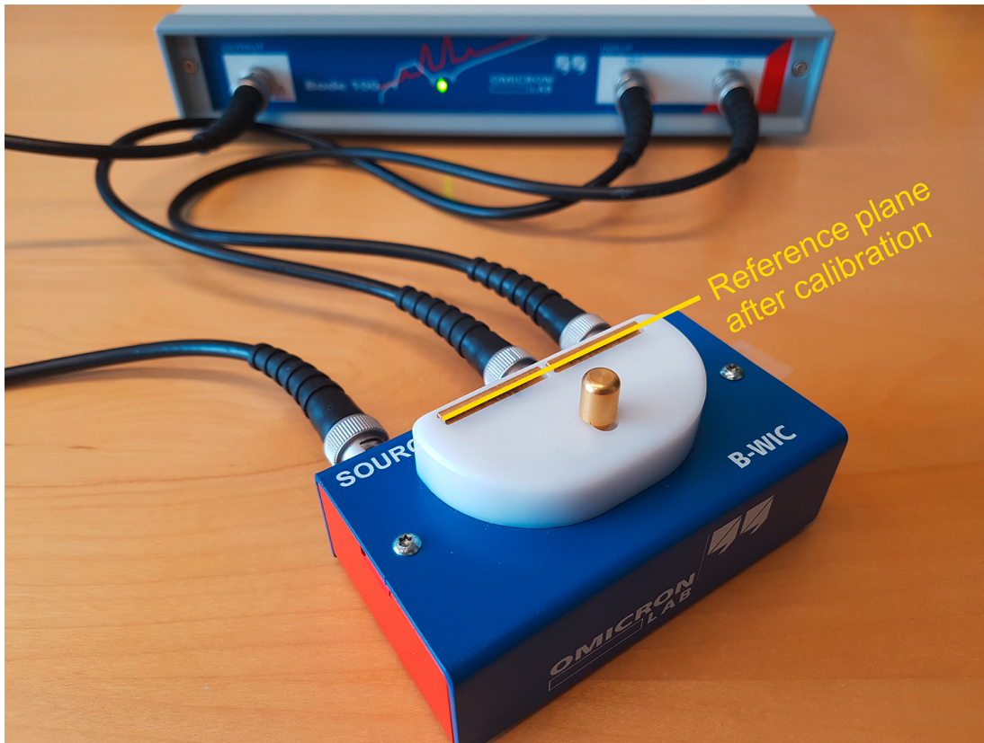
Figure 9-6: Calibrating the B-WIC impedance test fixture by performing Open, Short and Load Calibration
