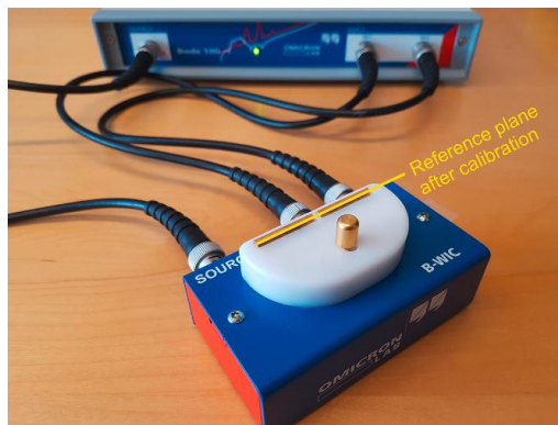
Figure 4-3: Reference plane after Open / Short / Load calibration
