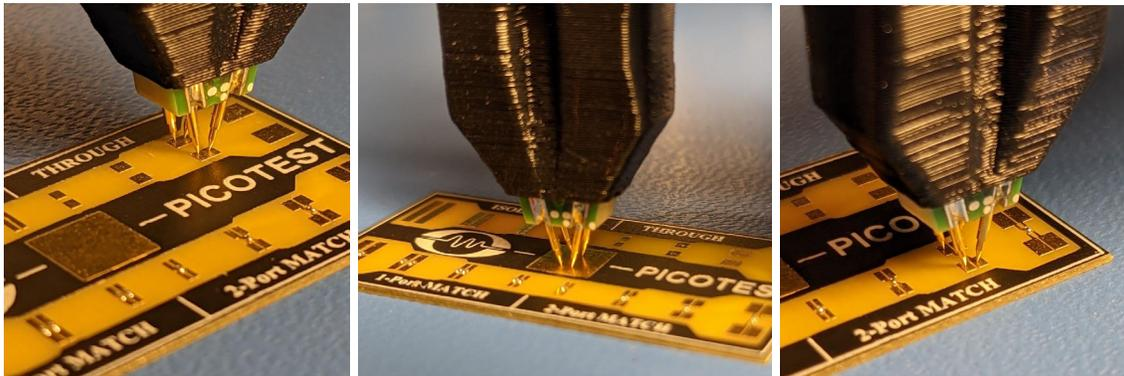
**Fig. 13 - P2102A 2-port Calibration Open (left), Short (center), and Load (right) with Bode 100.**
