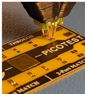
Fig. 12 - P2102A 2-port Thru-Calibration with Bode 100.
