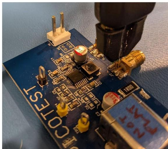
**Fig. 7 - Probe location on DUT - LM20143 at J2.**
