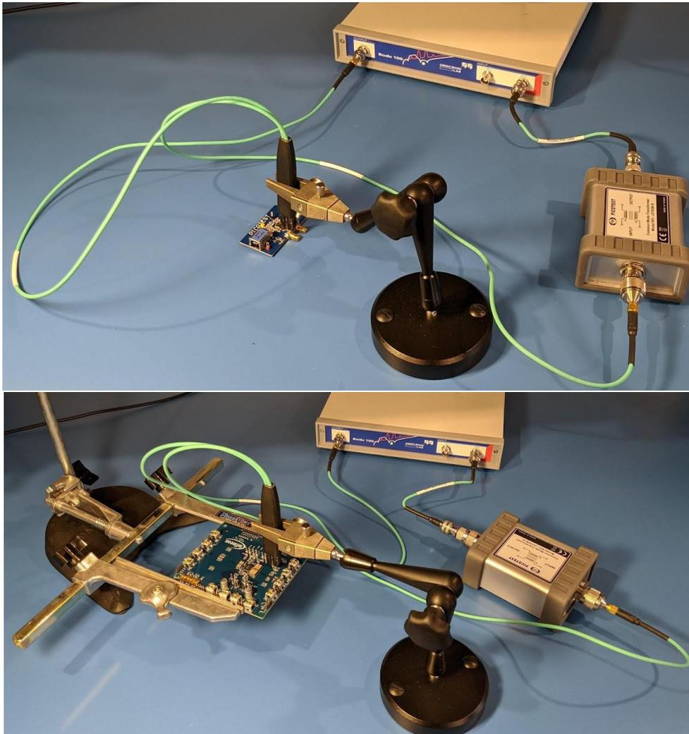
**Fig. 5 - Measurement Setup after Calibration with DUTs.**
