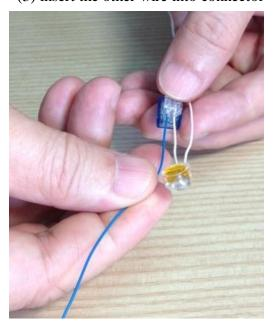
(5) Crimp connector for wire connection
