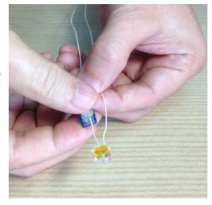
(4) finger press connector to fix the wire again.
