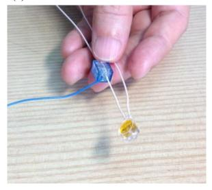
C. Application of UCC connector (a wire terminator for telephone wire)
