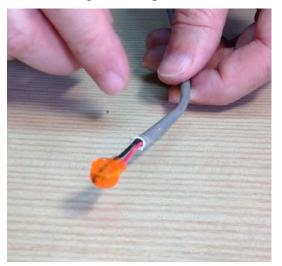
P.S.: The following picture display UCC does not have the "U Element" inside. The connector is mainly for insulation application ((i.e. water proof and prevent an electric shock) if the cable/wire are cut but without connection.
