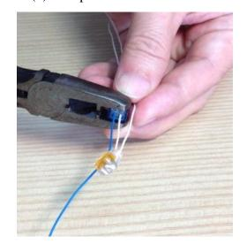
(2) finger press connector to fix the wire
