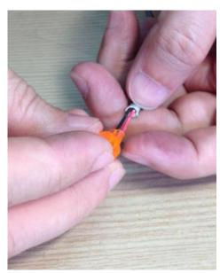
(3) Crimp connector to fix wires
